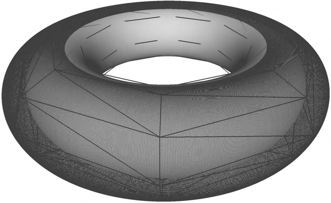
Figure 5.10: A fine triangulation of the torus (fine black mesh 1M faces ), a coarse triangulation of the torus (thick black mesh, 8 u- and 8 v-samples) and the Loop subdivision surface of the coarse triangulation (light grey faces).
